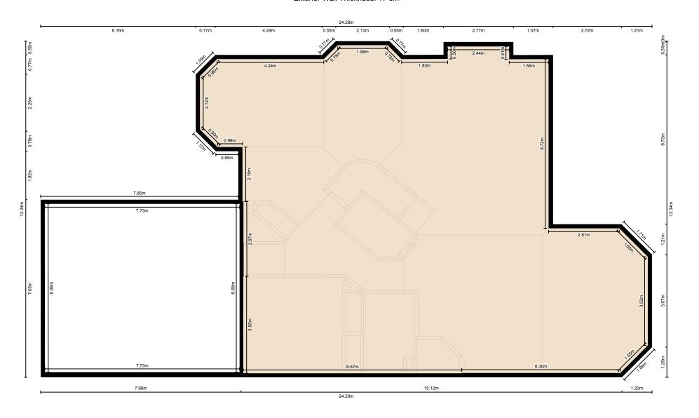
Measurement Diagram for: 2nd Floor Exterior Wall Thickness: 17 cm
