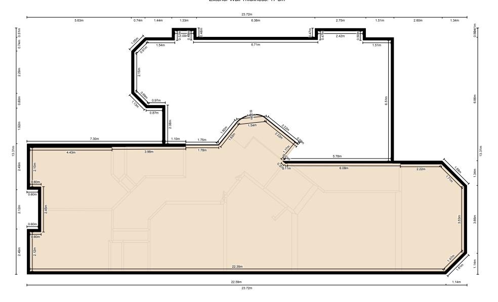
Measurement Diagram for: Basement Exterior Wall Thickness: 17 cm
